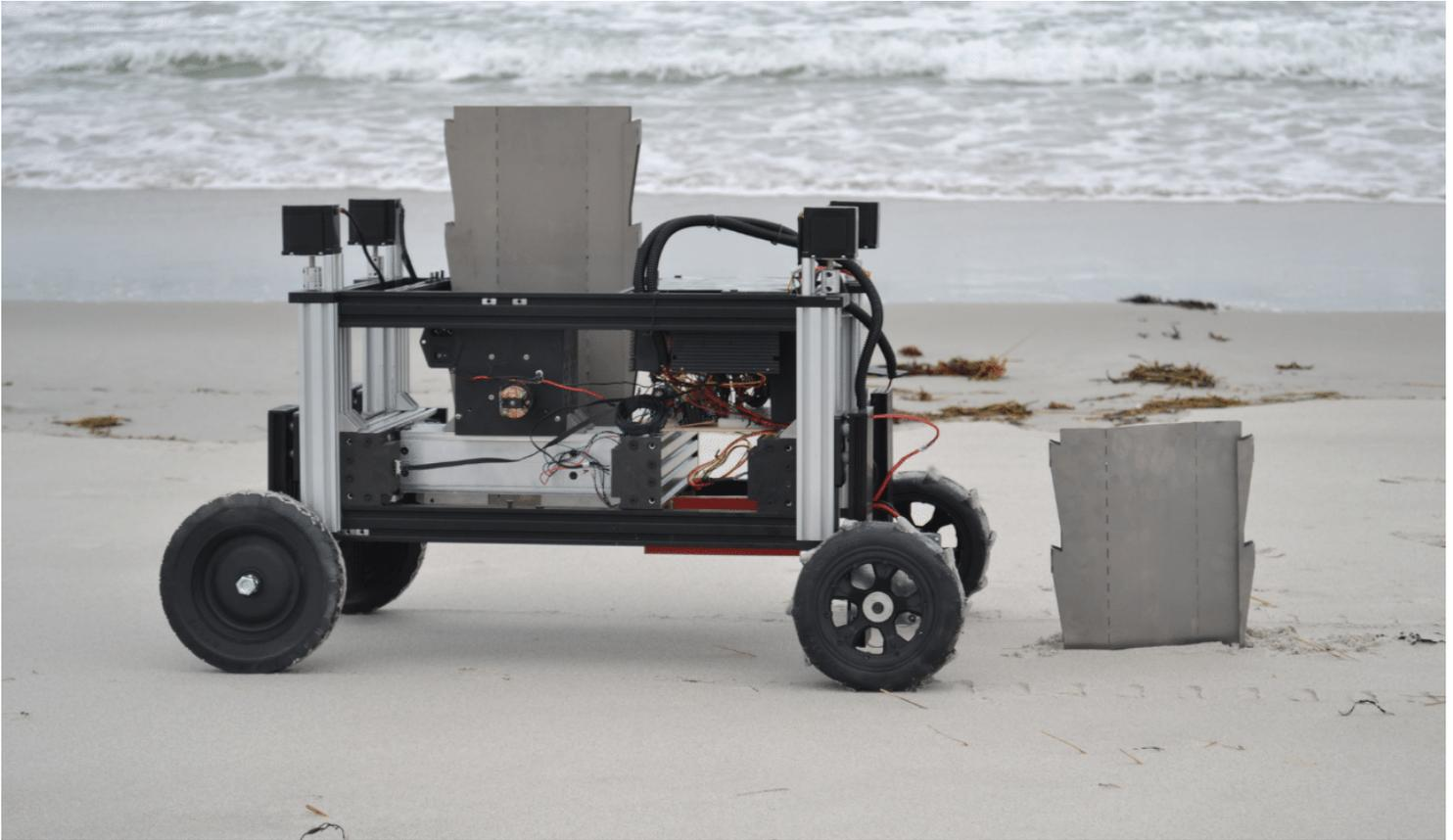
Romu can install erosion-minimising walls | Photo source [Wyss Institute at Harvard University](#)
