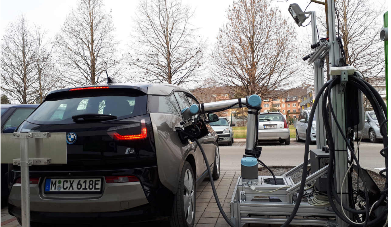
Robotic charging system
