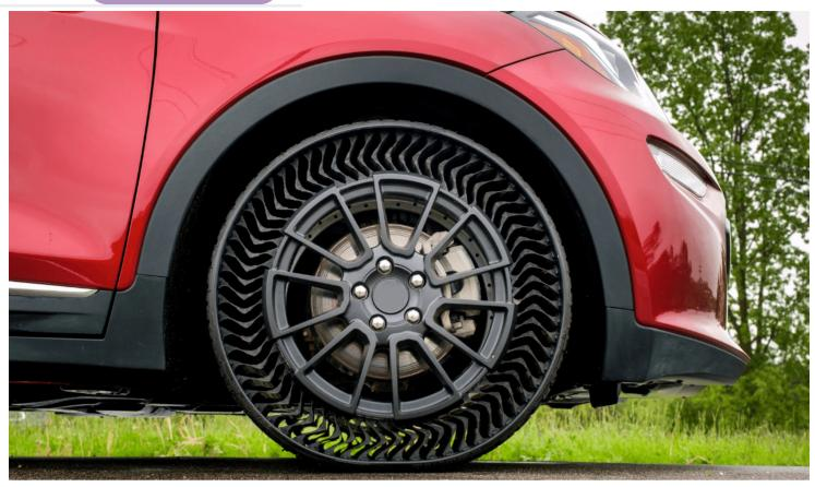
The airless tire can operate at highway speeds | Photo source Michelin
