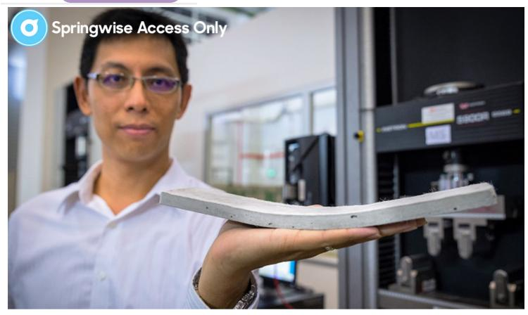
Innovation > Telecommunications > Easy upkeep, flexible concrete halves installation time
