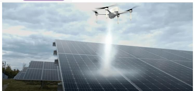
The new system uses a drone to automate the process of cleaning solar panels | Photo source Airobotics
