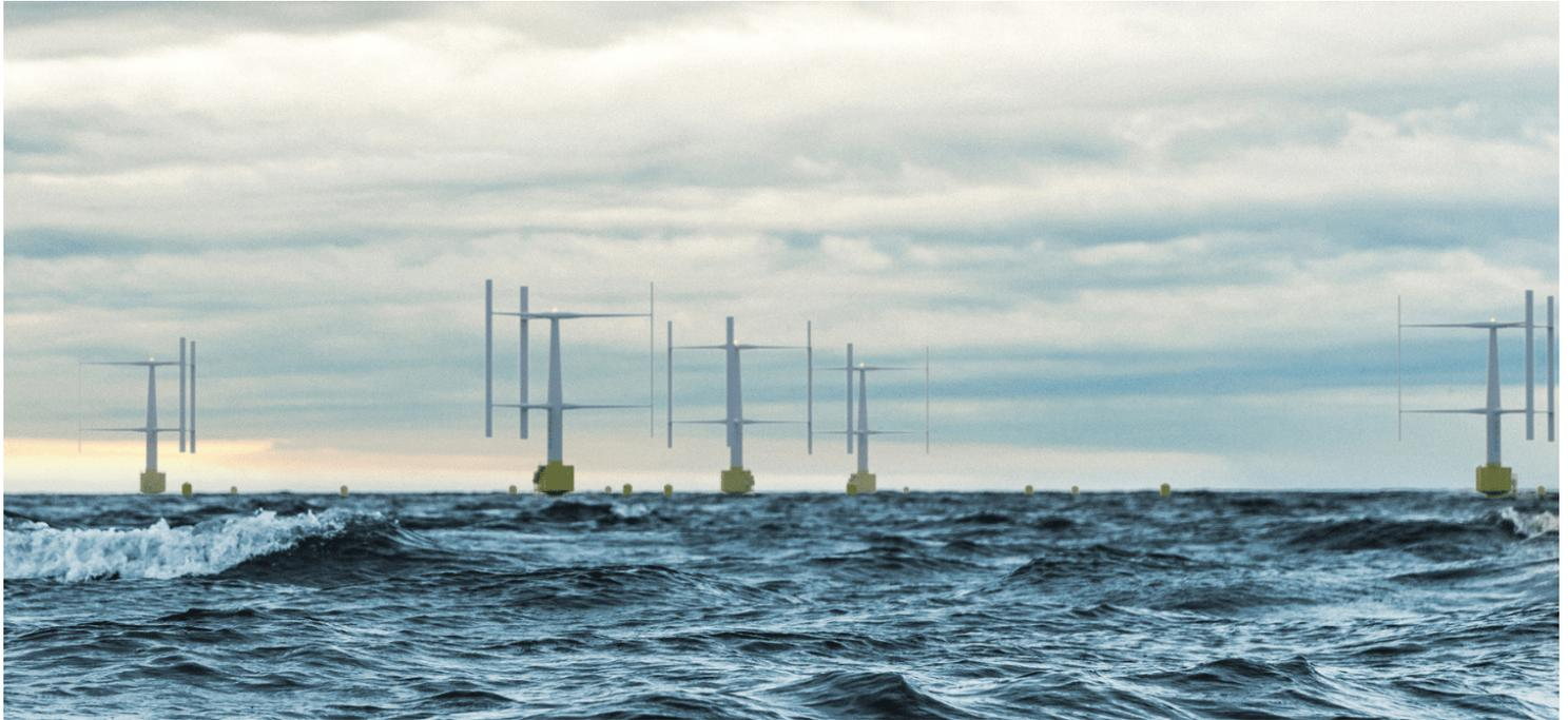
SeaTwirl is developing offshore vertical axis turbines | Photo source [SeaTwirl](#)
