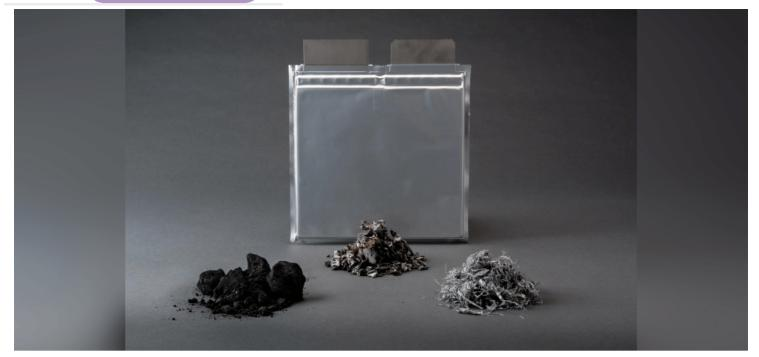
The adapted process uses froth flotation to separate battery materials | Photo source Argonne National Laboratory
