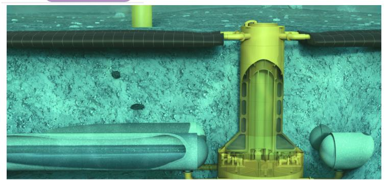
The Ocean Grazer storage system has a 70 to 80 per cent efficiency rate | Photo source Ocean Grazer
