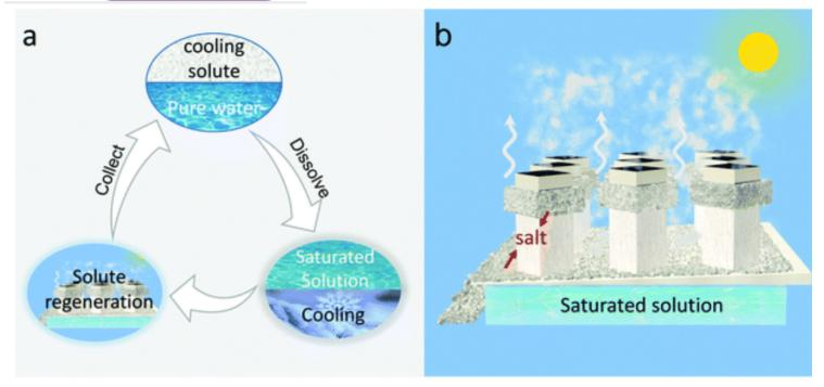
A schematic illustration of the no-energy, sustainable cooling on-demand system. (a) Cooling and regeneration cycle. (b) Solute regeneration. | Photo source Energy and Environmental Science / 3D SR
