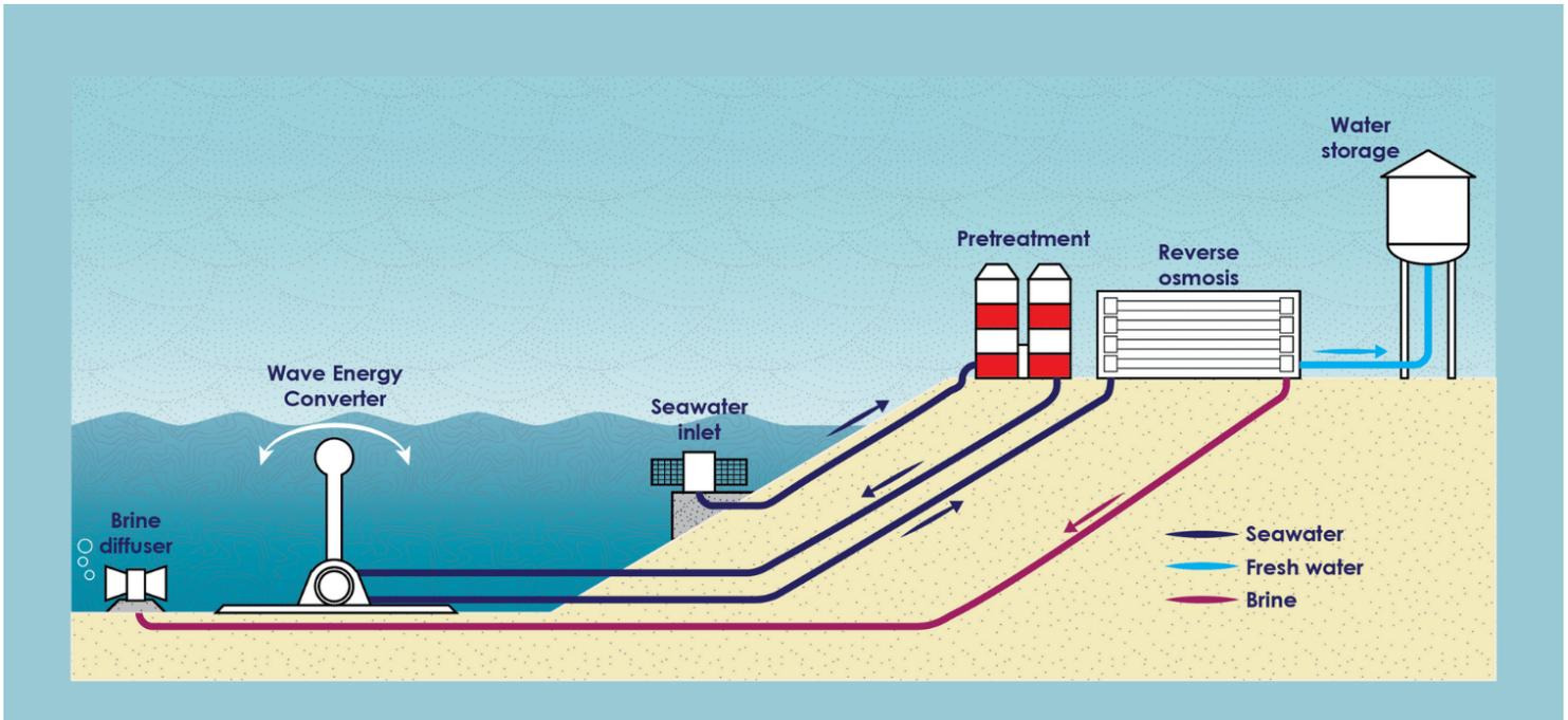
The new system uses the power of ocean waves to capture free energy for desalination | Photo source Resolute Marine
