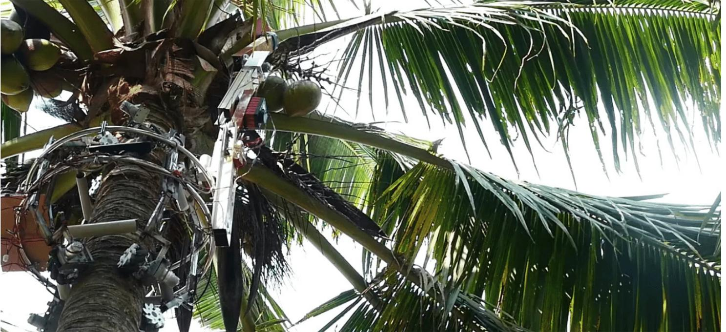
Amaran is able to climb to the top using its eight inward-facing omnidirectional rubber wheels | Photo source Amrita Vishwa Vidyapeetham University
