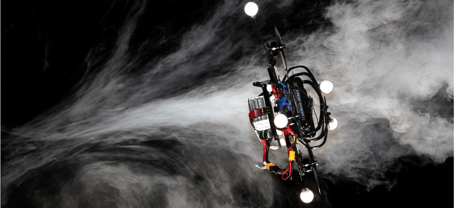
The winning drone used external cameras for real-time location information, allowing AI to plot the quickest route. | Photo source [Robotics and Perception Group, UZH](#)
