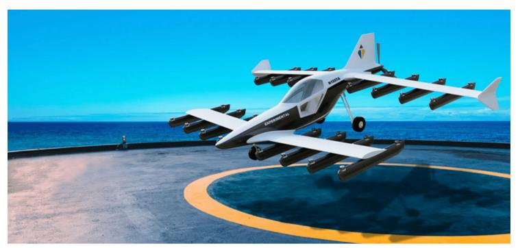
The lightweight planes hold a single person and are powered by 32 vertical lift motors. | Photo source teTra aviation corp
