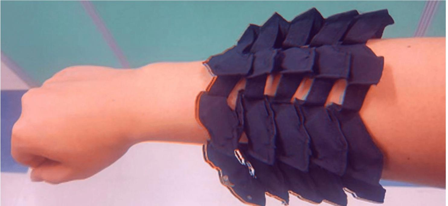
The shape of the battery minimises the deformation of the materials in order to ensure the battery's safety and give high capacity per unit size. | Photo source Korea Institute of Machinery and Materials (KIMM)
