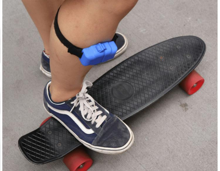
EmotiBit is a wearable open-source sensor for capturing high quality emotional, physiological and movement data | Photo source [Connected Future Labs](#)
