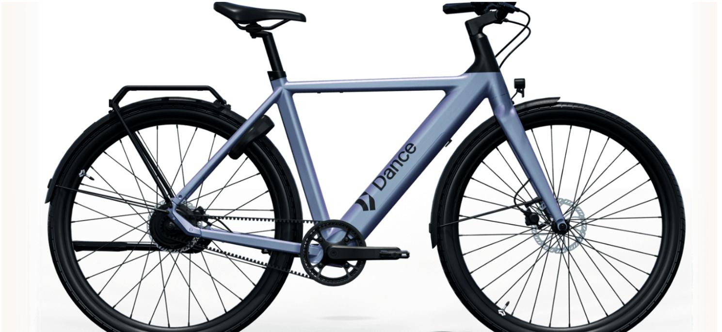
The Dance One's removeable battery can be plugged into any standard outlet, making it easier to maintain power between rides. The battery takes three hours to recharge and on a full charge, lasts up to 55 kilometres. | Photo source [Dance](#)
