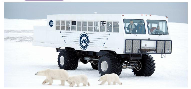
A repurposed battery from an electric bus makes the EV Tundra Buggy carbon-free as well as eliminating noise pollution. | Photo source Frontiers North
