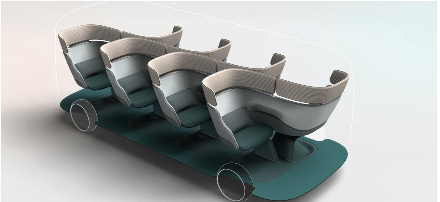
The Joyn vehicle consists of two rows of eight modular seats that are set in S-shaped pairs | Photo source Layer Design
