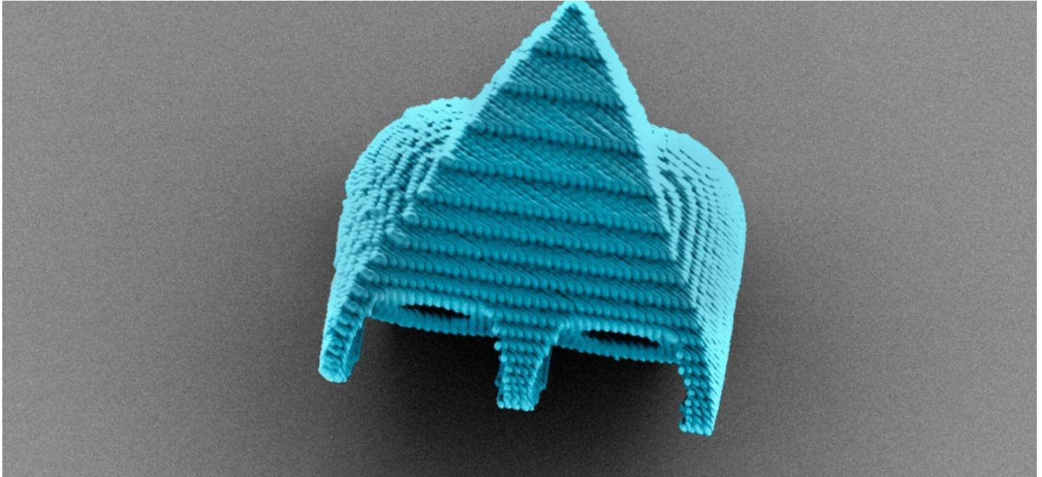
A scanning electron microscope image shows a cell-size robotic swimmer that can be powered and steered by ultrasound waves. | Photo source [Cornell University](#)
