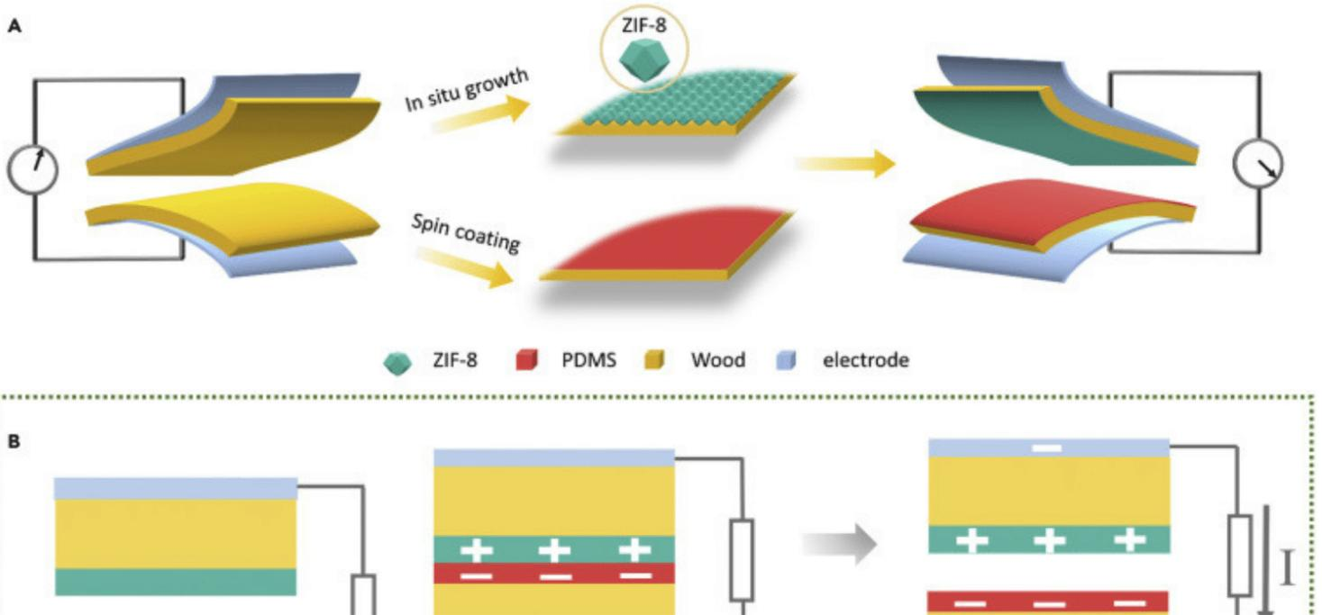
According to the researchers involved, the process caused the timber to generate electricity that was 80 times more efficient compared to natural wood. | Photo source Cell
