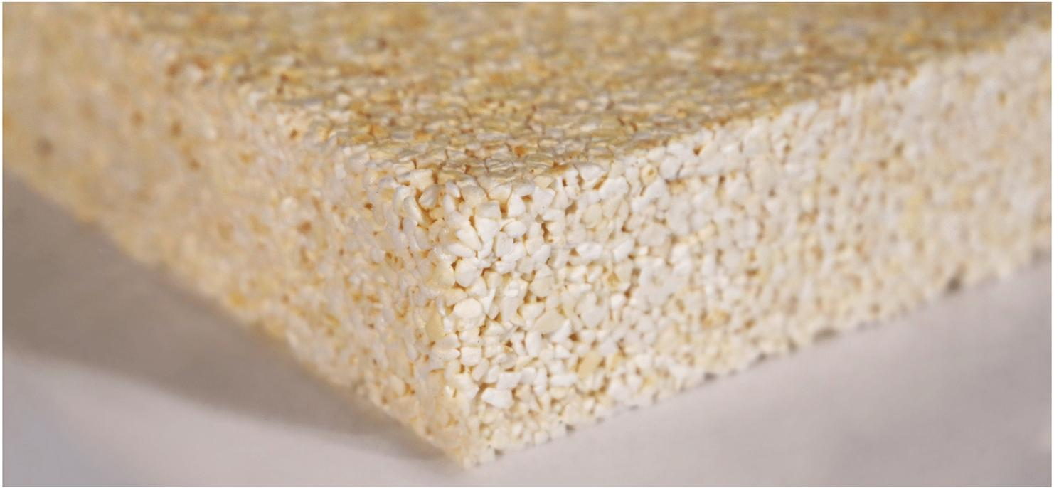
The popcorn-based insulation replaces the need for oil and mining | Photo source [Karl Bachl GmbH & Co. KG](#)
