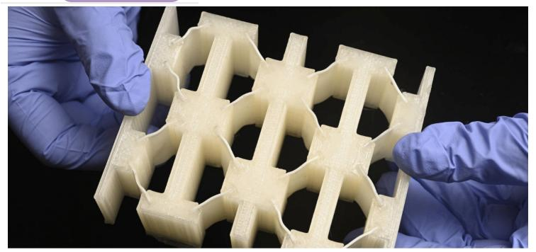
The material is built up out of layers of foam-like polymers | Photo source Will Kirk / Johns Hopkins University
