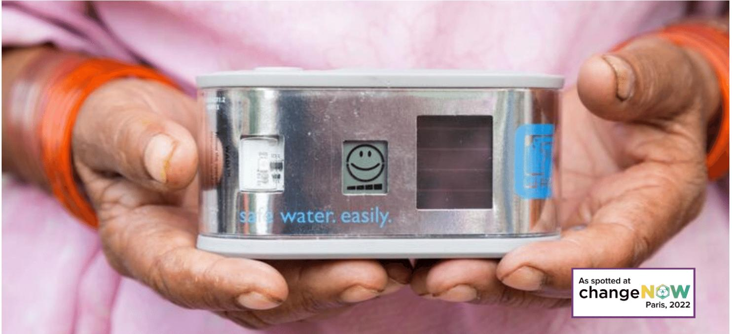
The WADI is a simple device that measures when contaminated water has been sufficiently exposed to sunlight to be safe to drink | Photo source [HELIOZ](#)
