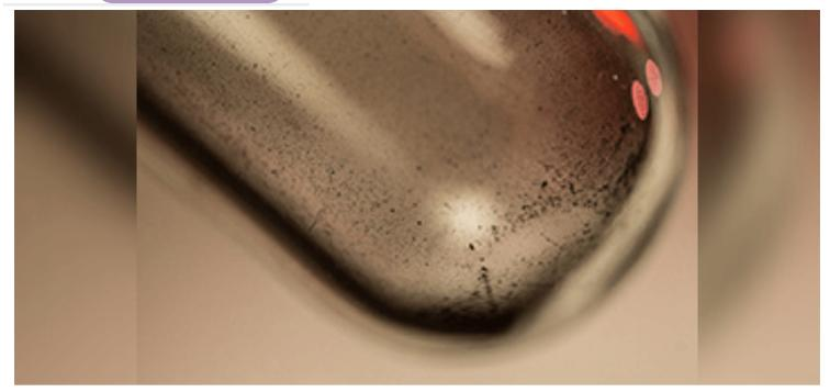
Metals settle at the bottom of the vial after being separated from other components in a crushed circuit board through flash joule heating. I Photo source Jeff Fitlow/Rice University
