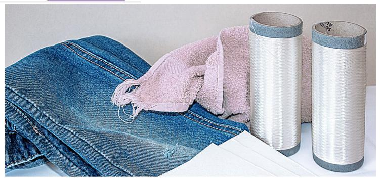
The viscose filament yarn made from recycled cotton | Photo source © Fraunhofer IAP
