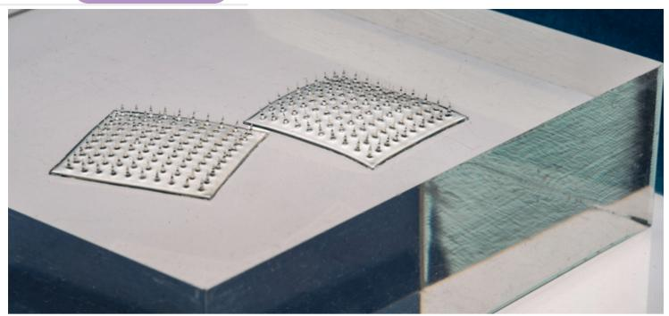
The Velcro-like food sensor, made from an array of silk microneedles, can pierce through plastic packaging to sample food for signs of spoilage and bacterial contamination | Photo source MIT / Felice Frankel
