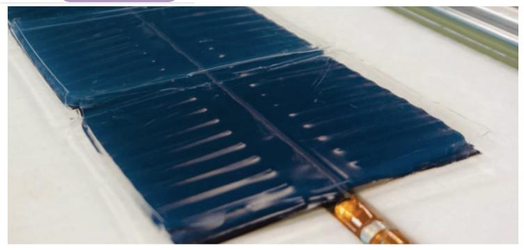
The aerogel-covered, black-coated copper plate | Photo source MIT
