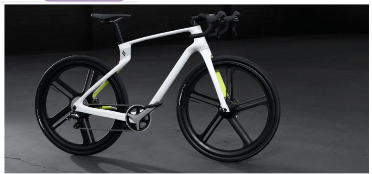
The Superstrata bike is made from a single piece of industrial grade carbon fibre | Photo source Superstrata
