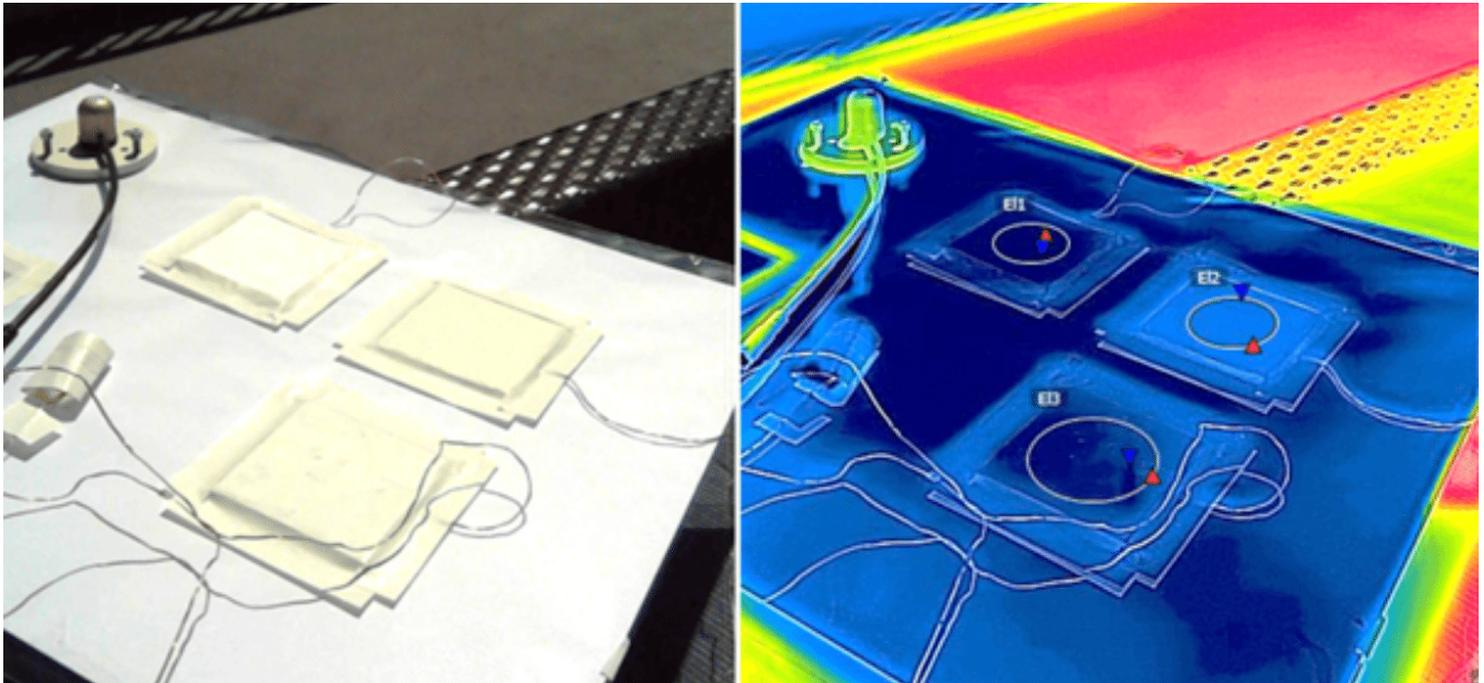
Under direct sunlight, superwhite paints developed by the researchers remain significantly cooler than traditional white paints, which could lead to higher energy savings in buildings | Photo source [Jyotirmoy Mandal](#)
