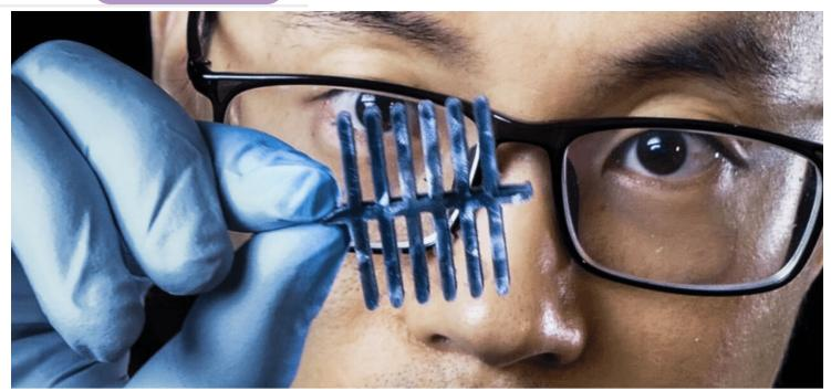
The sensor that can measure pressure, temperature and humidity simultaneously | Photo source Thor Balkhed
