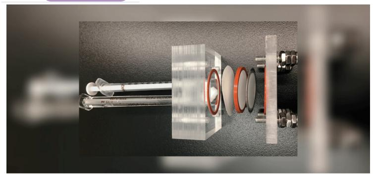
The device mimics the mangrove by more efficiently separating solutions and desalinating water | Photo source Yale
