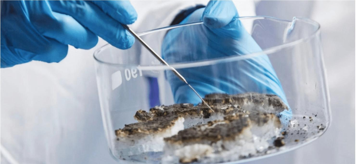
Successful in resisting temperatures of 1000 degrees Celsius for up to two hours, the fire-resistant glass meets current safety regulations | Photo source [Fraunhofer/Banczerowski](#)
