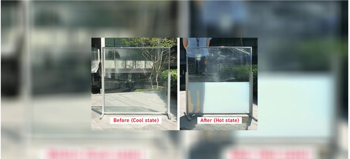
Photos showing the window in the before (cool) and after (hot) state | Photo source NTU
