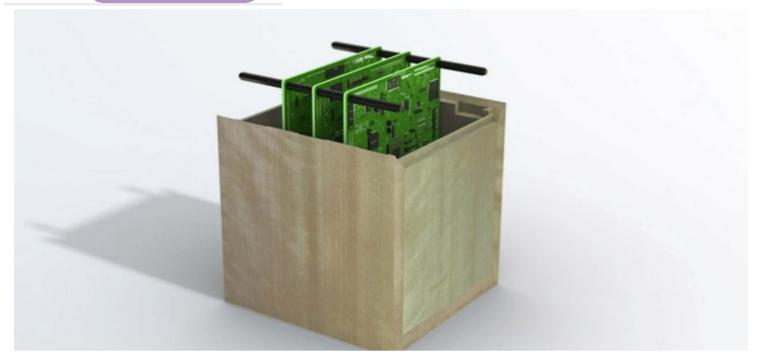
The wooden satellite shell is designed to burn up on re-entry, to minimise pollution and space junk | Photo source Sumitomo Forestry
