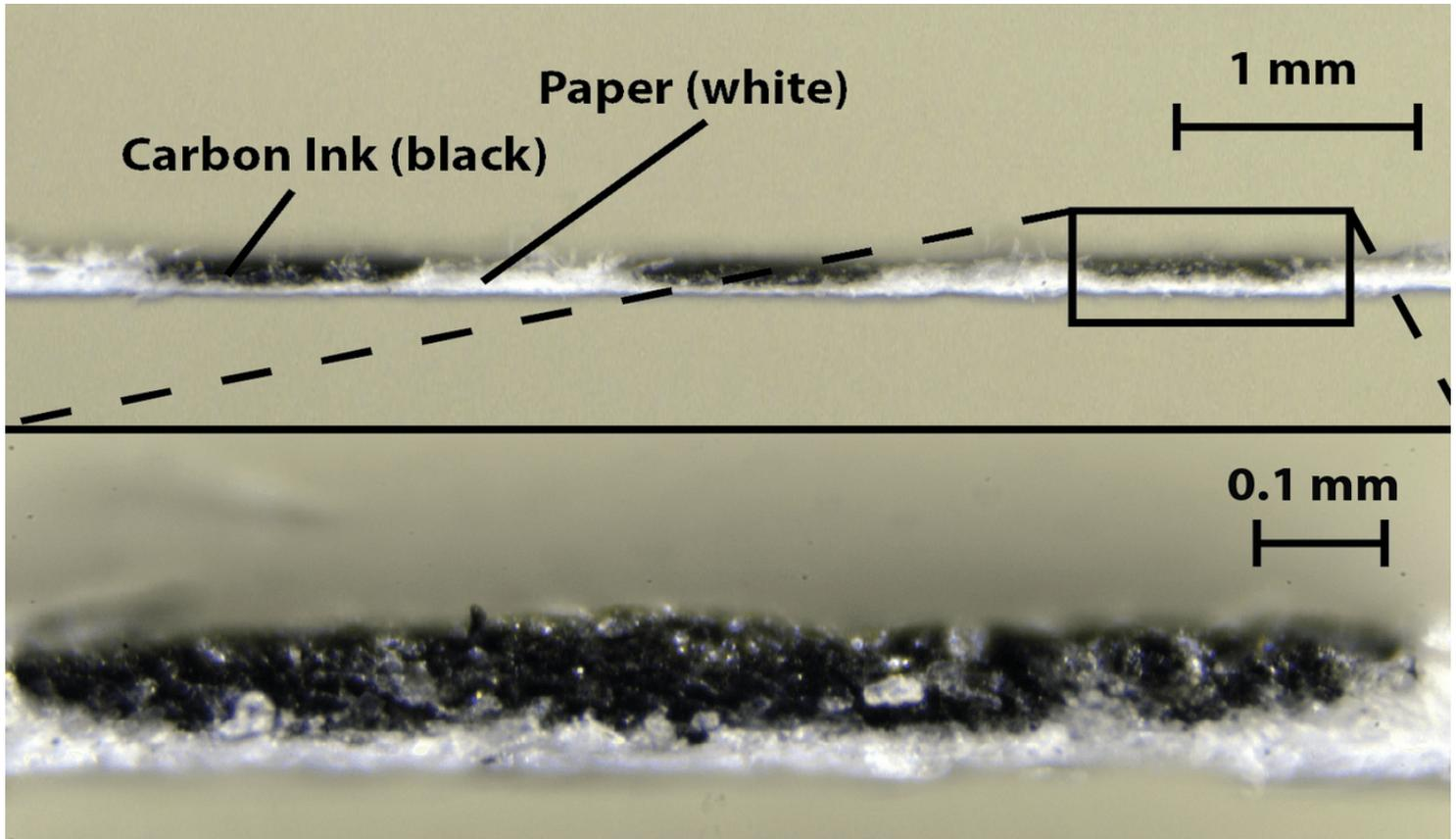
The sensors are made by printing carbon electrodes directly onto paper, making them biodegradable and non-toxic | Photo source [Department of Bioengineering, Imperial College, London](#).
